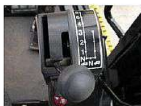
Full power shift transmission with torque converter
