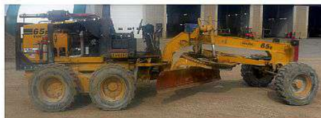
53" gear driven circle with "A" frame allows 360° blade rotation
