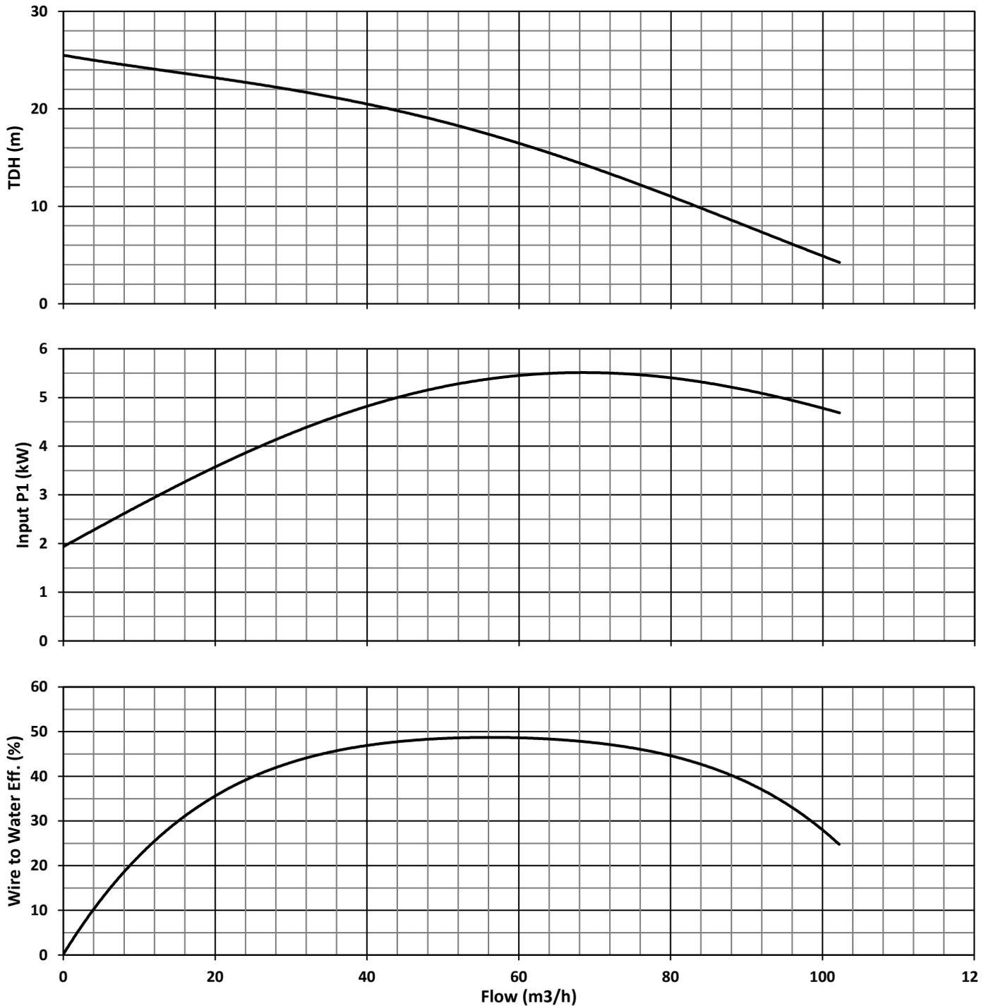
**Pump Performance Test - Metric Units**
