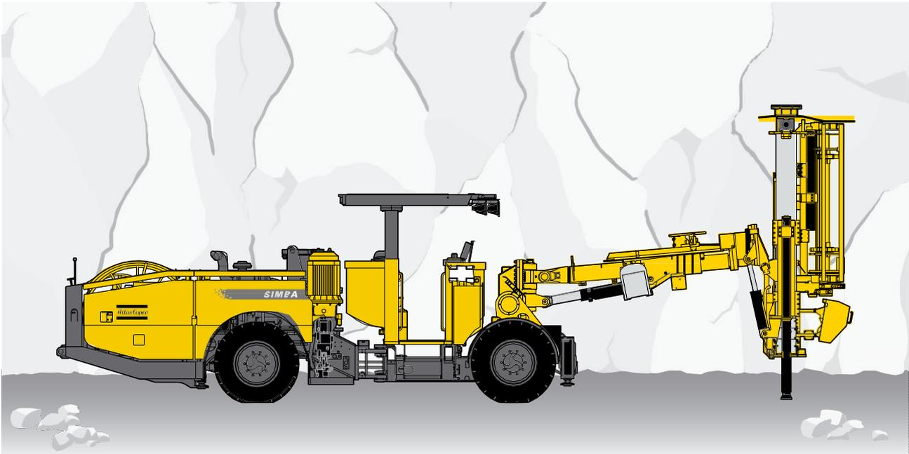
Long-hole drilling rig with top-hammer rock drill. The Rig Control System (RCS) provides efficient and high precision drilling, longer consumable life and an ergonomic working environment. Ring drilling with parallel holes upwards/downwards up to 5.5 m apart. Hole diameter 51–89 (102) mm.
