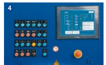
4 Control panel with GUI, positioned near the nozzleman/operator.
