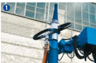
1 Modified MEYCO spraying head for 80 mm hoses and all required nozzle angles.
