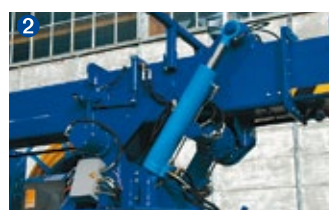
2 Ingenious construction allowing boom to be easily retracted for transport and extended for spraying.
