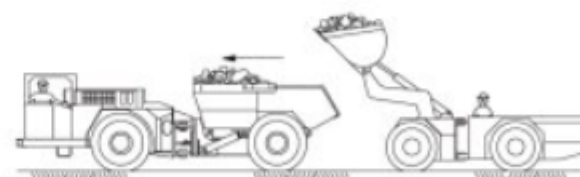
TELESCOPIC ACTION MOVES LOAD AHEAD
