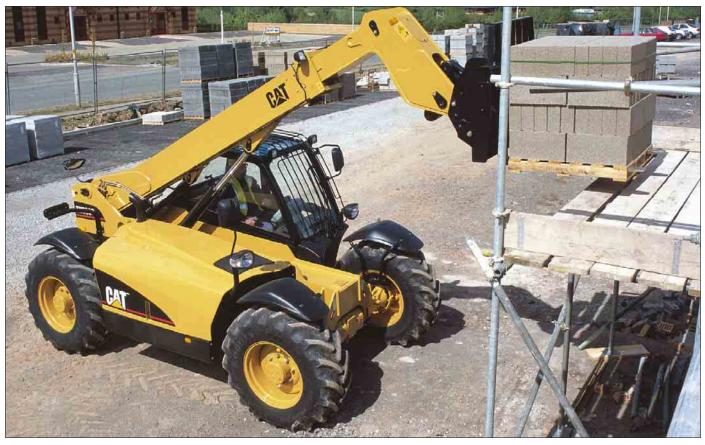
**Lift Height.** The TH330B can effectively and quickly place bricks, roofing materials and trusses to a maximum height of 7200 mm.
