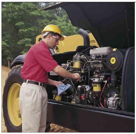
Access. All Cat Telehandler service points, including the combined transmission/hydraulic oil filter, are readily accessible and major components are easy to reach at ground level due to the overall machine design. A cab mounted service point allows access to the fuel fill, hydraulic oil fill, washer bottle, fuse box and cab air filter for daily checks.
