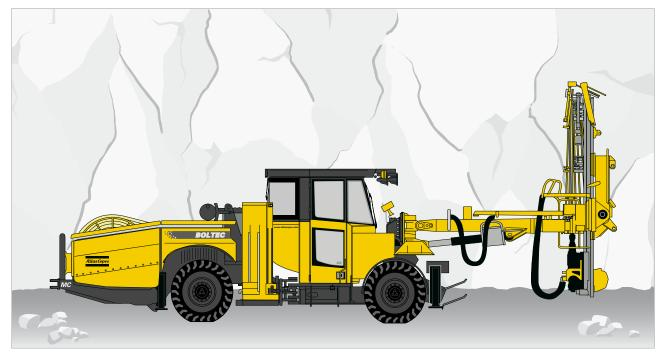
A fully mechanized rock bolting rig with RCS based control system for high productivity and precision. For bolt lengths 1.5–3.5 m and effective in roof heights up to 9.5 m.
